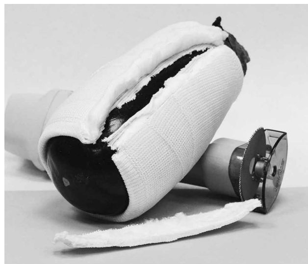
Figure 2 Eggplants were covered with fiberglass-casting material and cast padding and were used in the cast saw module.
